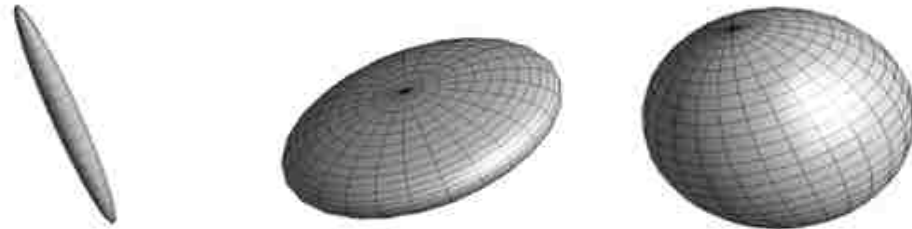
(a) Linear: \lambda_1 \gg \lambda_2 \approx \lambda_3 (b) Planar: \lambda_1 \approx \lambda_2 \gg \lambda_3 (c) Spherical: \lambda_1 \approx \lambda_2 \approx \lambda_3
